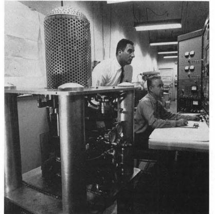
SANDIA PULSED REACTOR (minus fuel material) is shown at left while operators P. D. O'Brien and J. C. Conant (both 5431-2) are observing control console. The reactor will be located in a concrete hemispherical reactor building in Area III. This picture was taken in Bldg. 839 where the equipment was assembled.
